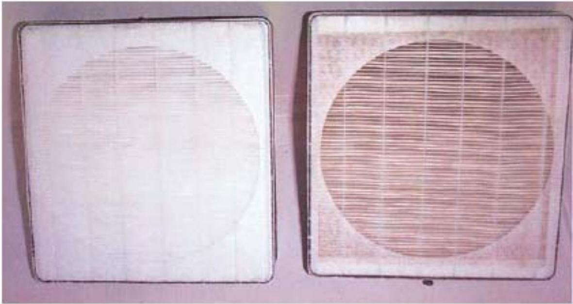
**Fig. 9 Examined filters. Left clean commercial filter; right Ecoservice filter following 20,000 page prints**
