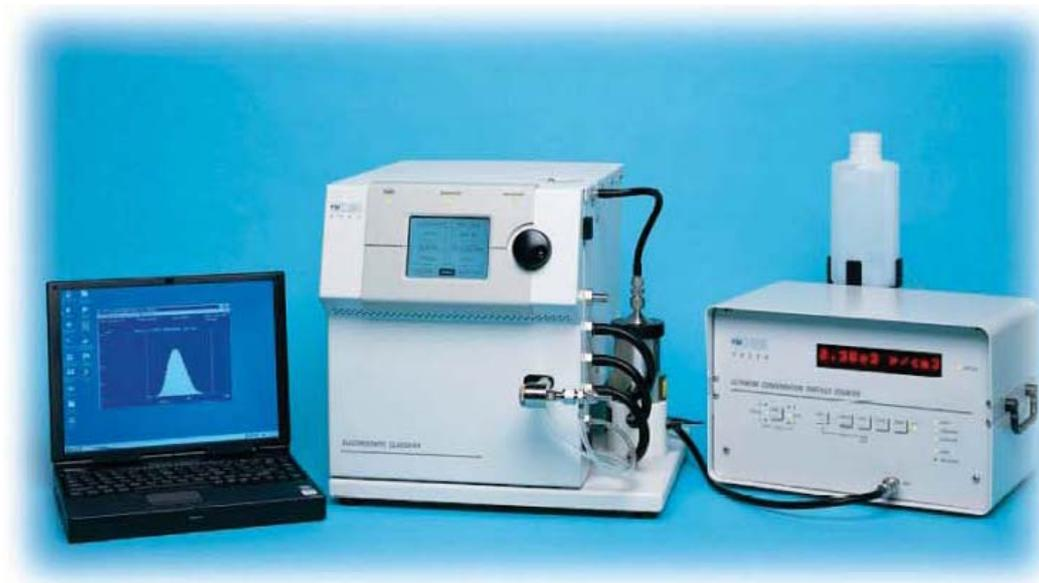
**Fig. 3 Scanning Mobility Particle Sizer Spectrometer**
