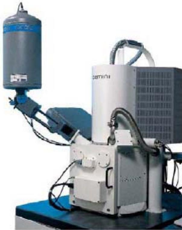
LEO SUPRA 50 with EDS detector installed.
