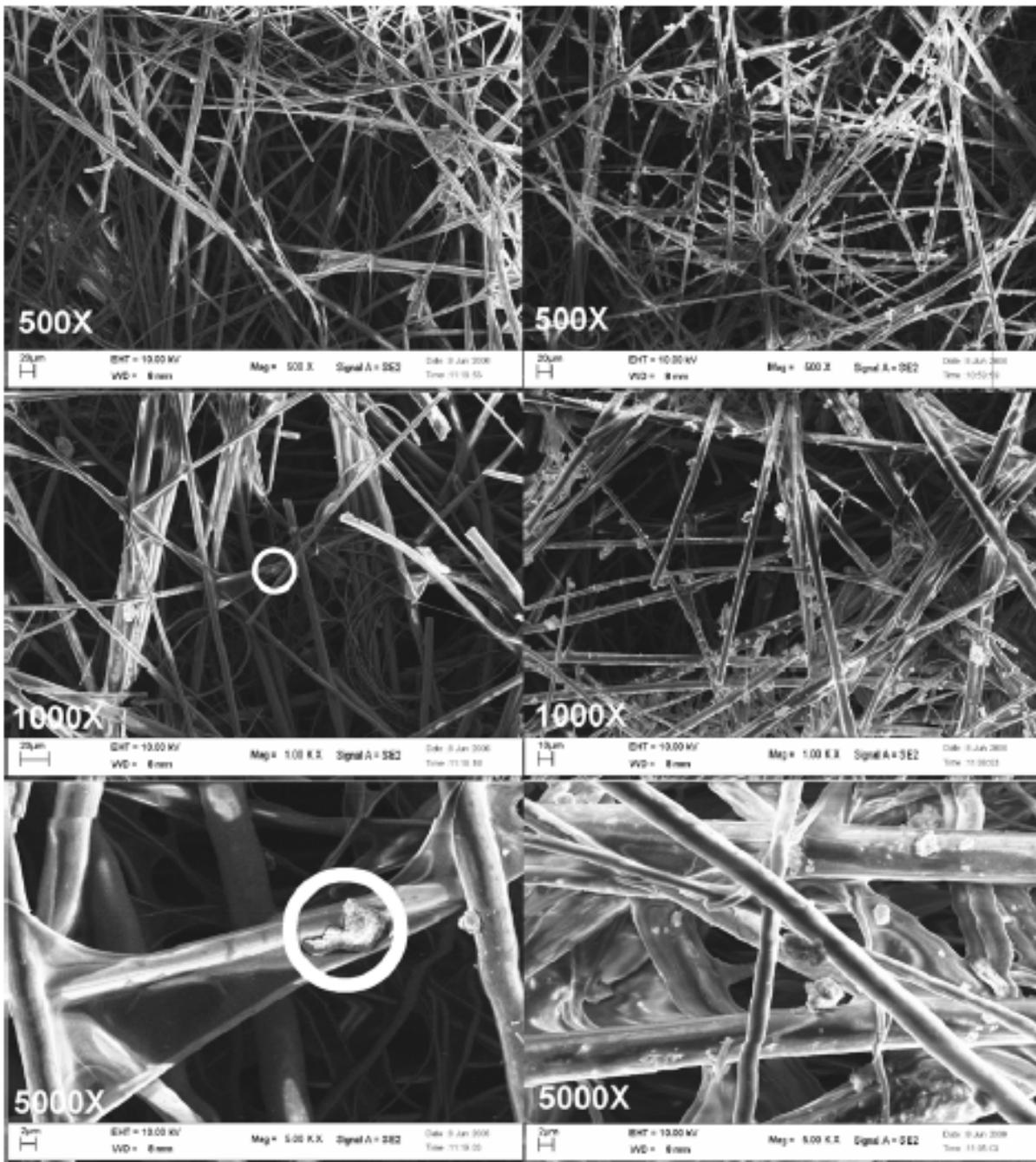
**Fig. 8 ESEM micrography: Enlargements 500 time, 1000 times and 5000 times. Left: an Ecoservice filter following 3000 page prints; right: an Ecoservice filter following 20000 page prints.**
