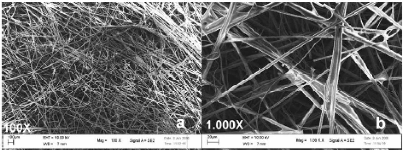
Fig. 7 FESEM Micrography with various enlargements (a) 100 times and (b) 1000 times of a clean Ecoservice filter.
