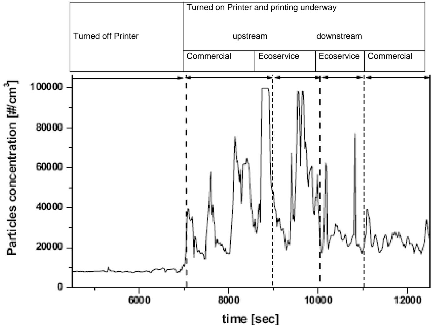
**Fig. 4 Mean Concentration of Particles between 2 and 1000 mm. First batch of trials.**
