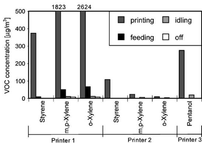
Fig. 9. VOC concentrations in the chamber on each printing condition.
