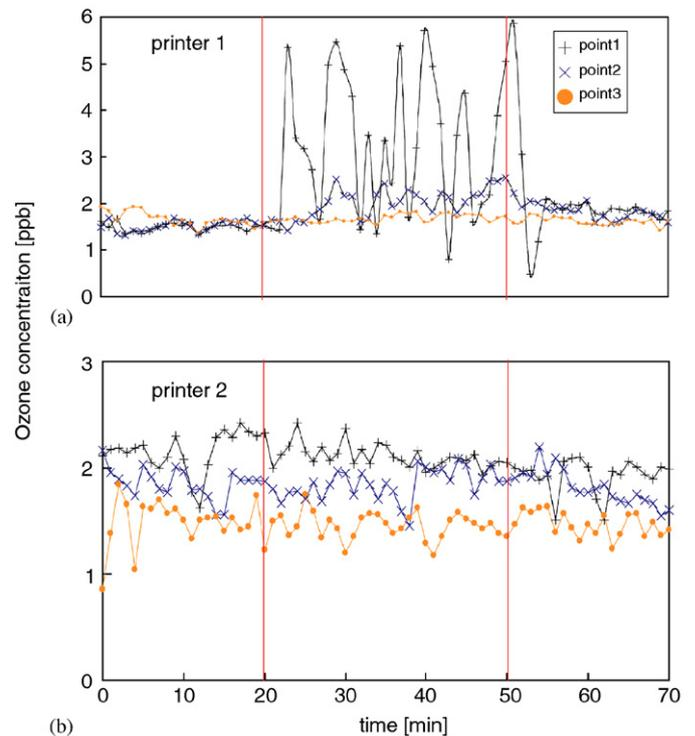
Fig. 2. Time variation of indoor ozone concentration for printer 1 and printer 2.
