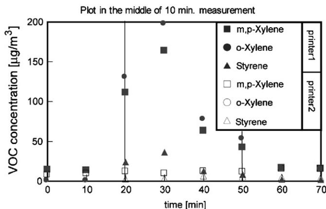
Fig. 5. Time variation of indoor VOC concentrations for printer 1 and printer 2.
