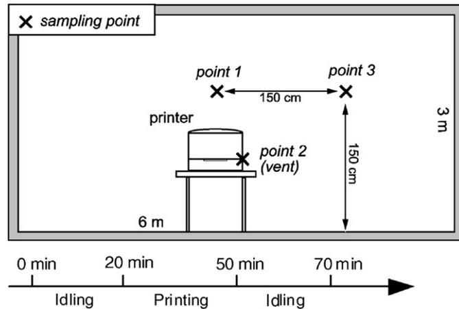
Fig. 1. Outline of measuring plan for indoor air measurement.
