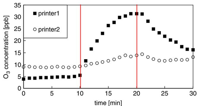
Fig. 7. Time variation of ozone concentration in chamber for printer 1 and printer 2.
