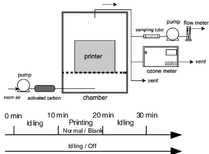
Fig. 6. Experimental apparatus and measuring plan for chamber test.
