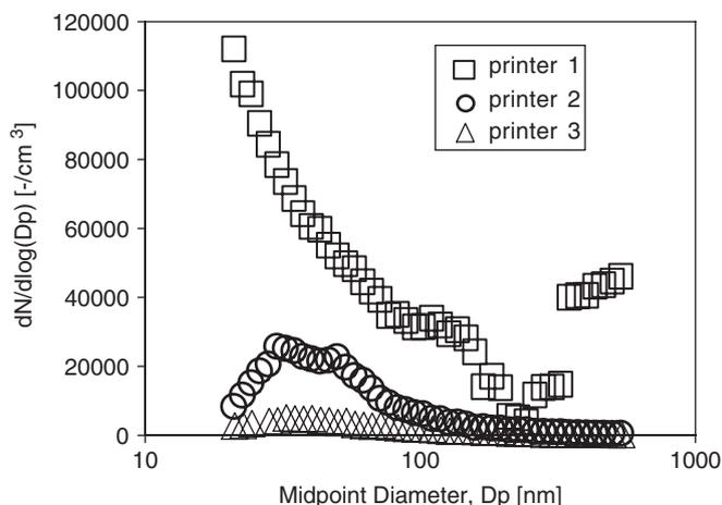
Fig. 3. Size distribution number concentration of particles at point 1 during printing.
