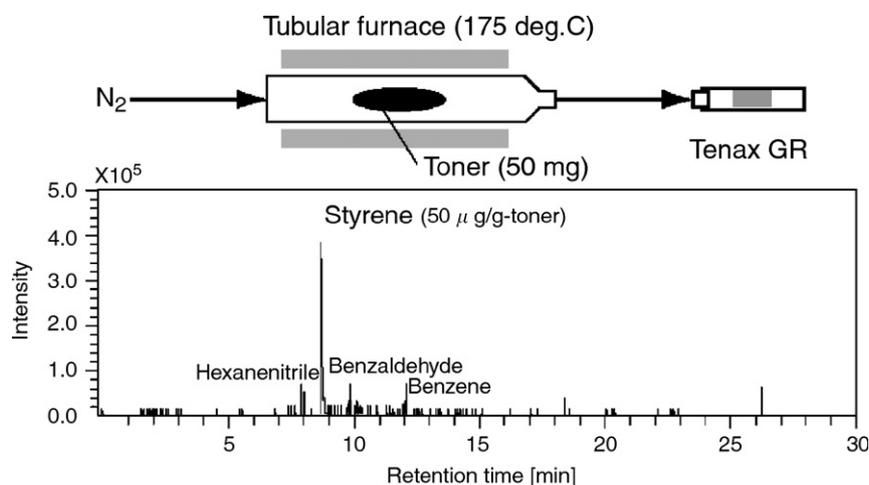
Fig. 10. Experimental apparatus and result of screening test for toner.
