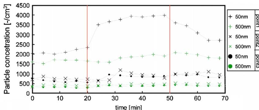
Fig. 4. Time variation of indoor particle concentration of 50 and 500 nm emitted from printer 1 at each point.
